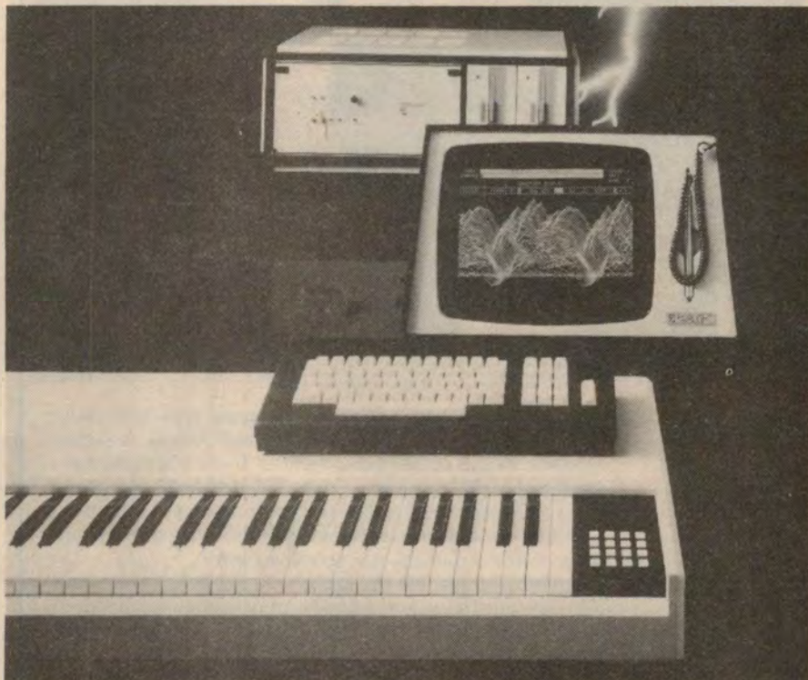
From the rear: the central computer unit including audio circuitry and floppy discs; the VDU with light pen; the computer style keyboard; the 6-octave music keyboard. The small numeric key pad at the front-right can be used as a tone selector — in the manner of organ stops — for stage performances.
