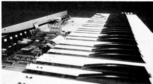
The master keyboard with its own processor can calculate the velocity of any key depression
