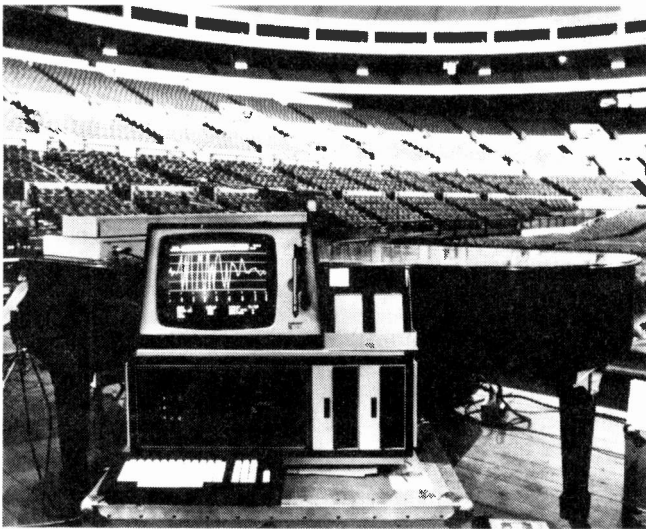
Entire musical scores can be fed into the computer via the VDU's alphanumeric keyboard
