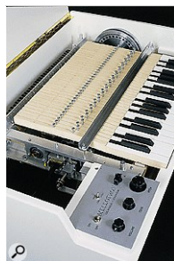
Flipping the lid of the MkVI open reveals the keyboard frame. The track-selector mechanism can be seen in the bottom left of the picture, located behind the front-panel controls on the unit.
