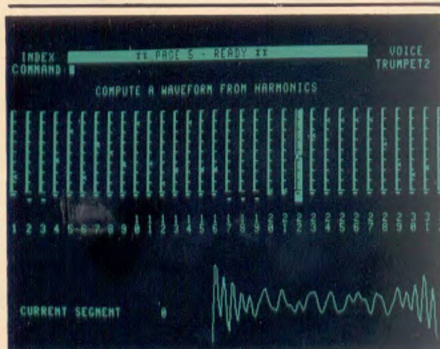
WAVEFORM FROM HARMONICS: A single cycle of waveform is displayed as its constituent harmonics are specified by setting a series of "slide pots" with the light-pen.
