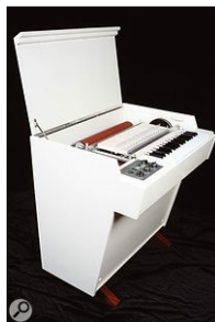
Lifting the lid on the M4000 reveals the keyboard mechanism and a glimpse of the tapes themselves.
