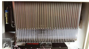
With the front cover off we can see the tape return springs and also the Filtron unit at the bottom of the case.
