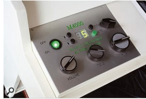
The M4000's control panel: identical to the M400's, aside from the addition of four buttons and an LED display to operate the cycling mechanism.
