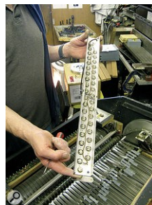
The head block. You can see some of Robert Webb's splices on the tapes below.
